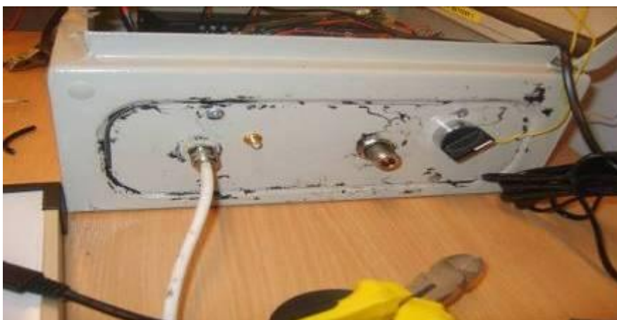
FIGURE 8 FINISHED GLAND PLATE
