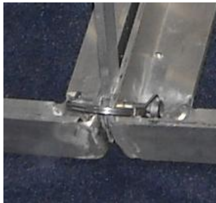
FIGURE 25 CLOSE UP OF LEG WITH CLIP
